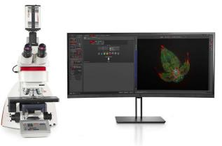
acquisition of different fluorochromes (24 ms filter change speed between adjacent positions)
