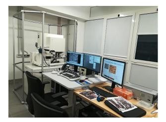
The wide range of detectors with which the FEG-SEM is equipped makes it an extremely powerful instrument for the characterization at a submicroscopic scale of synthetic materials, and geological and biological samples.
